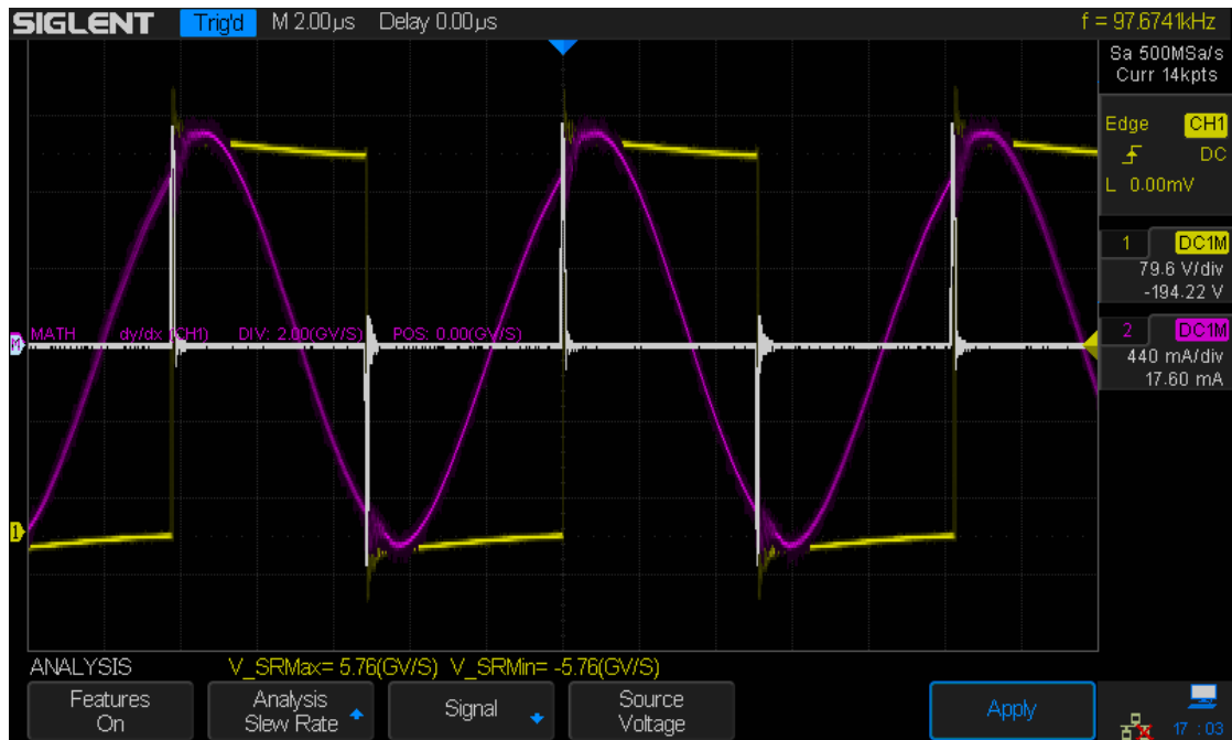
Figure 117: Perform Slew Rate Analysis
