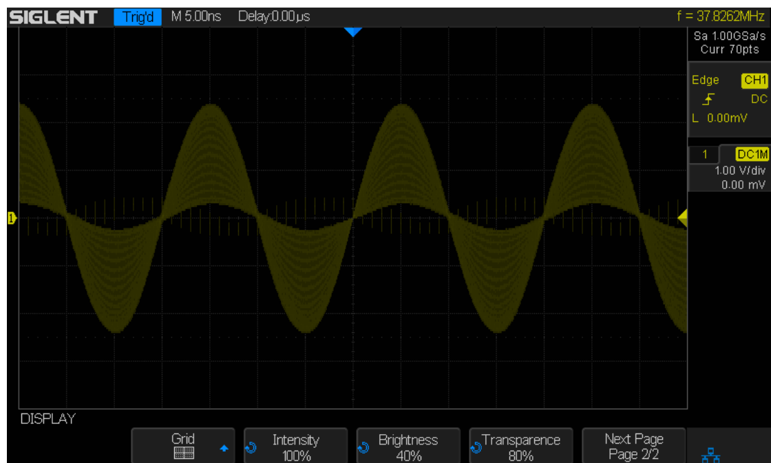
Figure 85: Intensity Set to 100%
