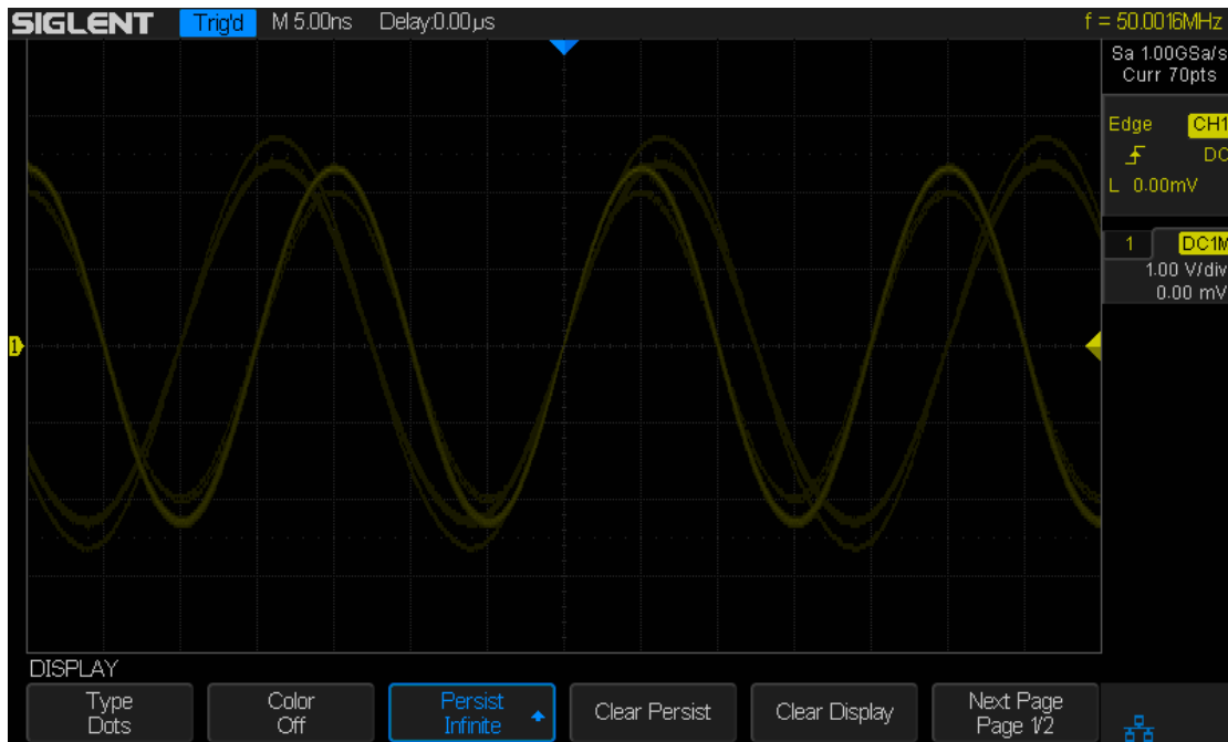
Figure 84: Persist Set to Infinite
