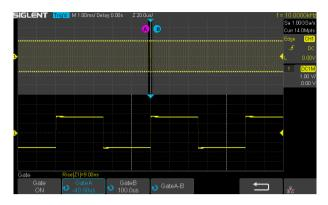
Through Gate and Zoom measurement, the user can specify an arbitrary interval of waveform data analysis and statistics. This helps avoid measurement errors that can be caused by invalid or extraneous data, greatly enhancing the measurements' validity and flexibility.
