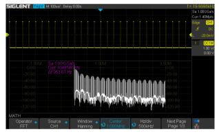
The new math co-processor enables FFT analysis of incoming signals using up to 1M samples per waveform. This provides high frequency resolution with a fast refresh rate. The FFT function also supports a variety of window functions so that it can adapt to different spectrum measurement needs.
