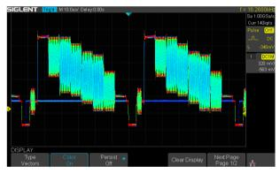
The color temperature display is similar to the intensity-graded trace in function, except that the trace occurrence is represented by different colors (color "temperature") as opposed to changes in the intensity of one color. Red represents the most common occurrences or probabilities, while blue is used to mark points that occur least frequently.
