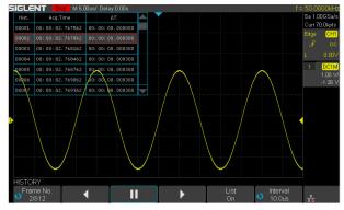
Playback the latest triggered events using the history function. Segmented memory zcquisition will store the waveform into multiple (up to 80,000) memory segments, each segment will store triggered waveforms and timestamp each frame.
