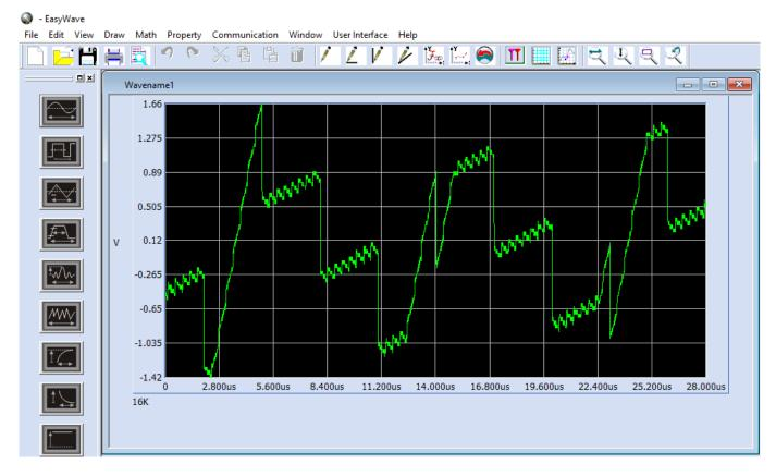
9. Select Communication > Send Wave to pass the waveform to the scope generator memory:
