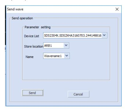
12. The waveform should now be stored in the AWG memory of the scope. You can check it by accessing the AWG menu by pressing WaveGen button on the front panel, select the Waveform Type and File:
