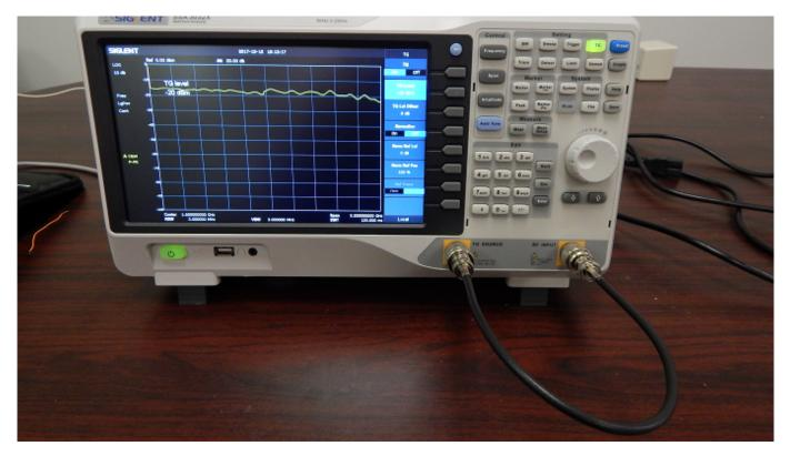
Connect a cable from the TG output to the RF input and enable the TG:
