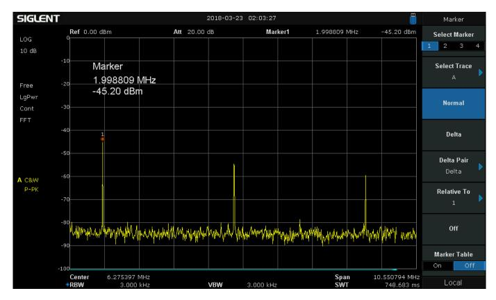
As you can see, there is now a marker at 1.998809 MHz with an amplitude of -45.20 dBm.
