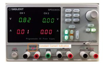
Note that with no load attached, the supply still indicates that the output is in constant current mode. This is a false indication due to the incorrect value of the MAINS input selection switches.
