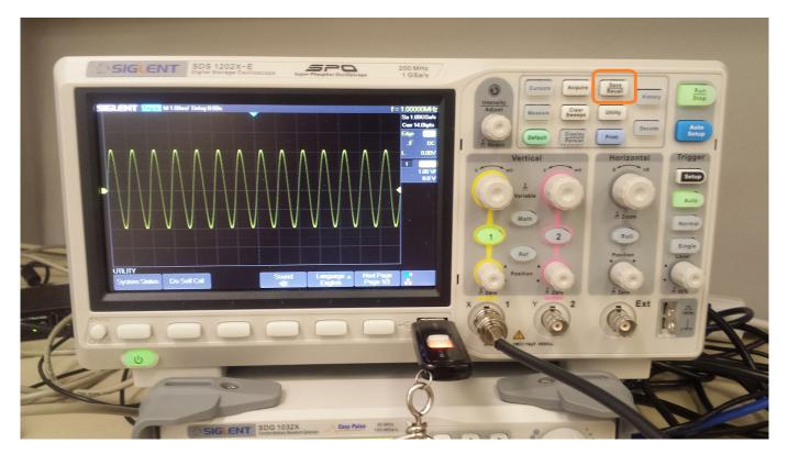
3. Press the softkey located below the "Save" label to open the Save menu
