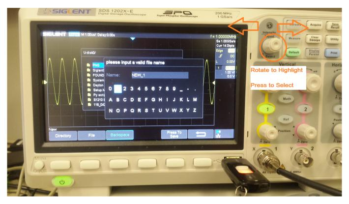
For example, you can press backspace to remove all of the default file character names, then use the intensity/adjust knob to highlight "N", and press the knob in to select the character as shown:
