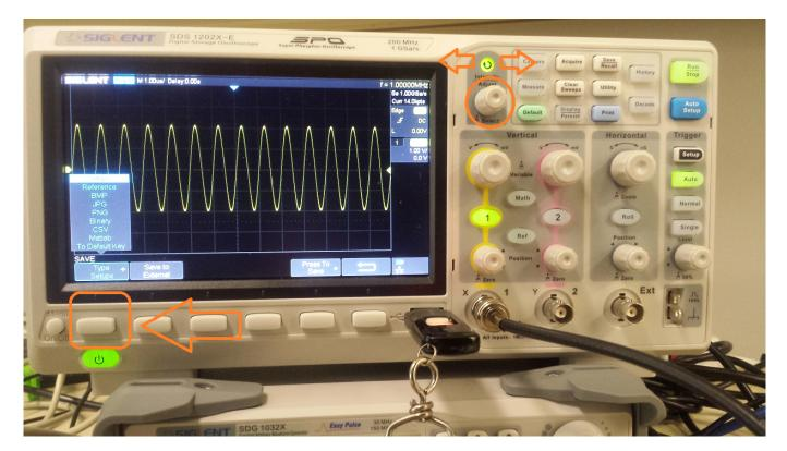
5. Set any additional options (Screen type, Parameter Save, etc..) to configure the instrument to properly save the information that is of interest to you.
