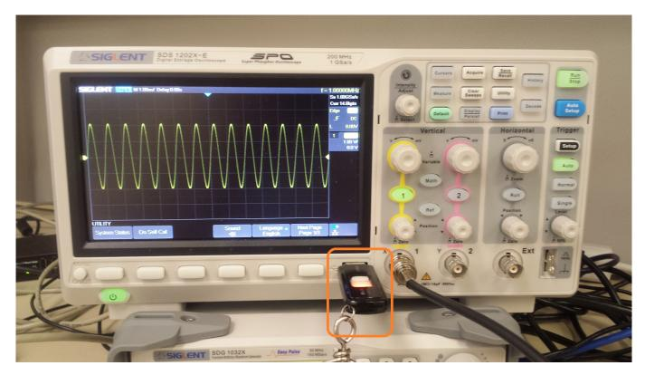
If the USB Memory device is recognized, a USB shaped icon will appear on the display, as shown below:
