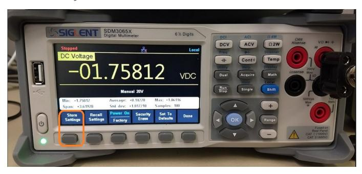
9 Set current Path to External by pressing Browse and use the Up/Down range arrows to highlight 'external' and press select. External will only appear when a USB memory stick (FAT32 format) is inserted into the front panel USB slot.
