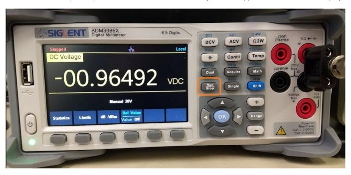
2. Clear the memory buffer by pressing Math > Statistics > Clear Readings (The number of stored samples is shown next to the Samples label)
