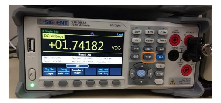
5. Wait for data buffer to fill (STOP on the DMM display is displayed and the sample number should equal to the setpoint in step 3)
