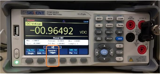
4. Press the "Single" button to start the acquisition. When the meter is collecting data, there will be a flashing green dot and the word "trig" on the display. The sample count will also increment as each measurement is completed.
