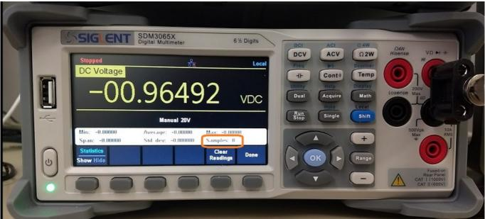
3. Press Acquire and set the sample/trigger to the desired number. In this example, we are going to set the sample count to 100 using the Up/Down/Left/Right keypad. NOTE: Left adds decimal places, right subtracts. Up adds digits and down subtracts them.
