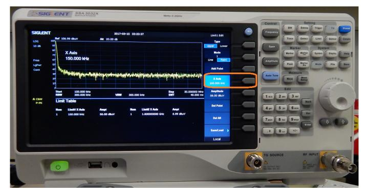
7. Press the grey colored soft key next to the entry labeled Amplitude and enter the Average start amplitude, 56 dBuV. If using a Quasi-peak detector, use the Quasi-peak values of the chart.
