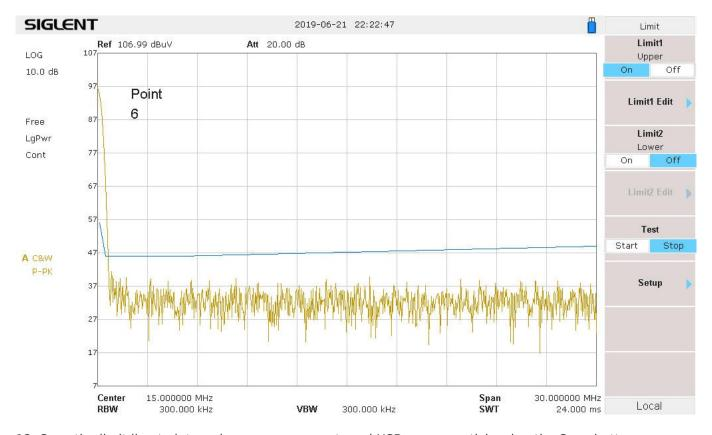
12. Save the limit line to internal memory or an external USB memory stick using the Save button
