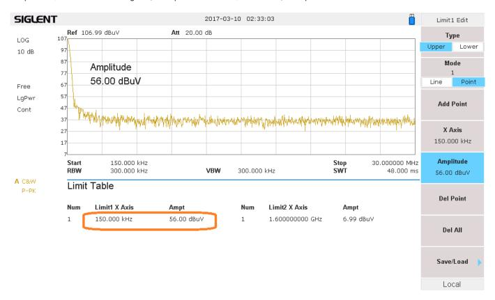
8. Press Add Point and enter X Axis and Amplitude values for the second point, 500 kHz and 46 dBuV. Now,
