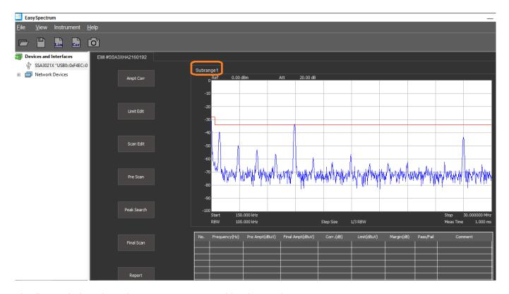
The figures below show the same span covered by three sub-range segments:
