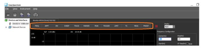
**FREQ:** Set the start, stop, center and other frequency and span parameters
