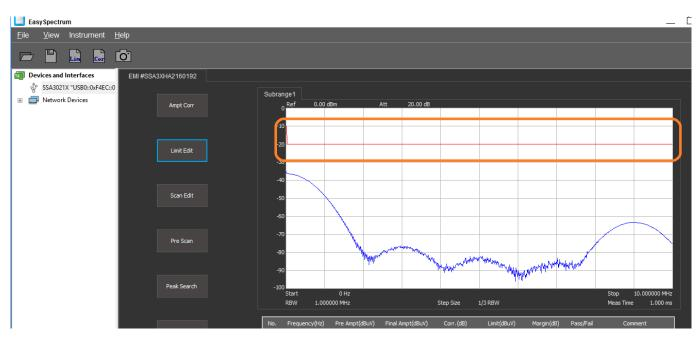
5. Scan Edit: Configure the scan which is broken up into three distinct parts. While they can be configured in many different ways, here are oursuggested settings for preliminary scans:
