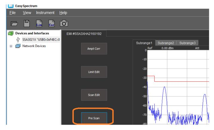
The figures below show a pre-scan configuration consisting of a single segment from 150 kHz to 30 MHz and the subsequent scan data:
