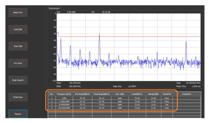
The peak table shows the frequency, pre-scan amplitude, final scan amplitude, the limit at that frequency, the margin between the peak and the limit, and the pass/fail of that peak based on final scan data.
