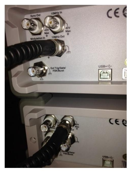
The next step is to set Unit 2 so that it uses the external 10 MHz time base (from Unit 1).
