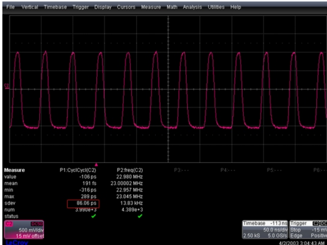
P4 EasyPulse waveform with low jitter
