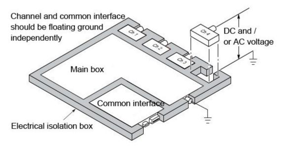
There is no real ground reference level of a handheld oscilloscope. As shown above, the ground reference for the various modules belongs to virtual ground, and the reference voltage of the oscilloscope channel directly relies on the input voltage of the probe's clip.
