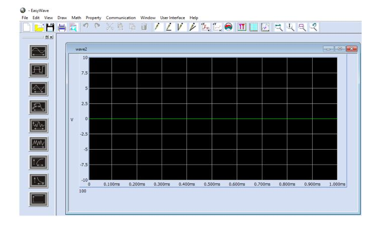
• Save the file as a CSV by pressing File > Save As > set the file location and name. If you are using an SDG2X, you can also directly open the SDG2X template file that is available with this application note
