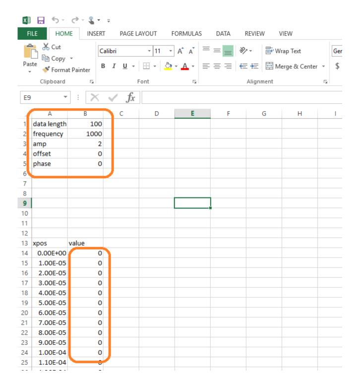
• After you have built the waveform, save the Excel file as a CSV. Use a specific name to indicate the waveform type and output sample rate or another useful identifier.
