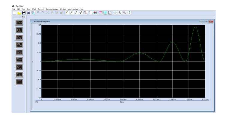
Now, download the file to the instrument. The front panel of the AWG will indicate that the waveform is an ARB and will have a picture representing the new waveform on the front panel:
