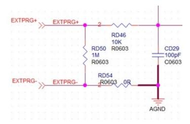
7. What is the input resistance (impedance) for each of the "+" and "-" inputs?
