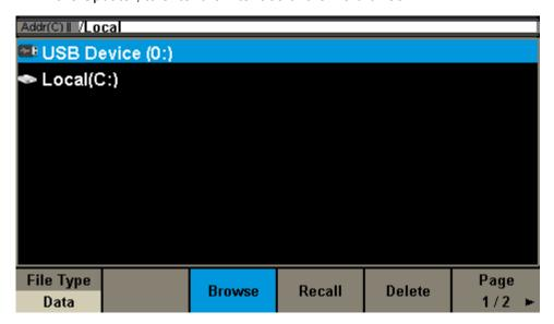
3. Select "USB Device" thru the knob on the front panel, press "Browse", and then select the correct ads file using the knob
