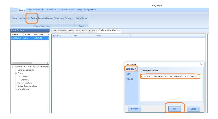
4. Configure the instrument to capture the signal of interest. You can perform this manually on the front panel, or you can use the Virtual Panel control.
