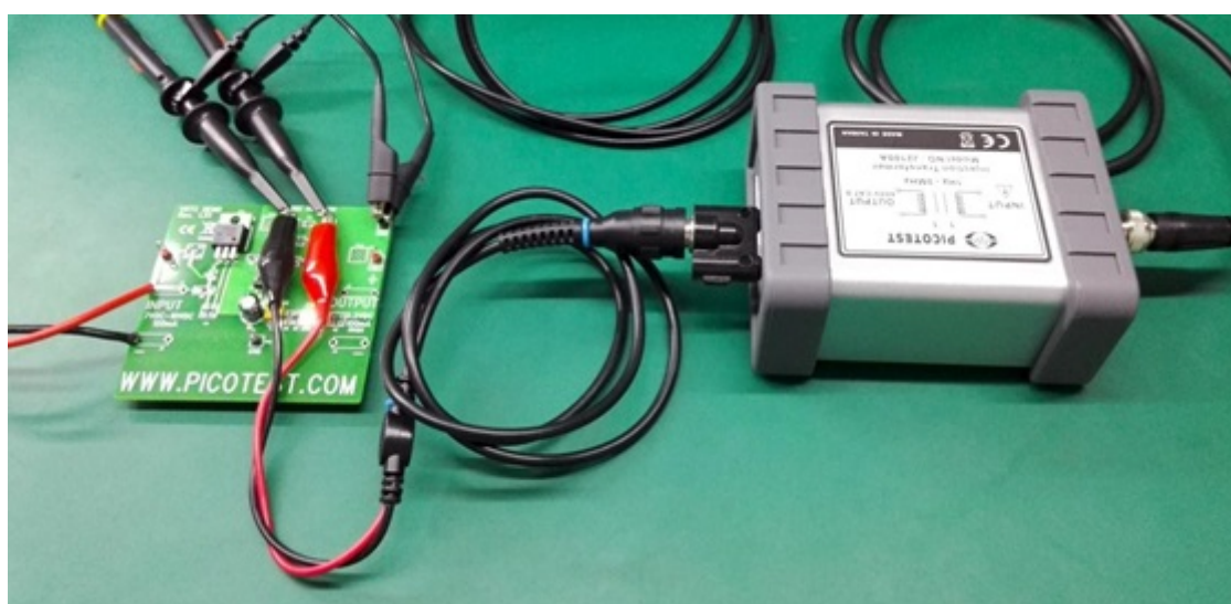
Figure 9: Probe and Transformer connections to the DUT
